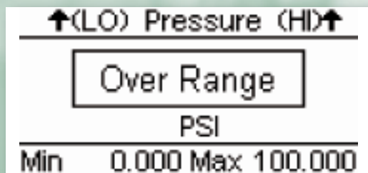
Typical display with "Over Range" message box.
